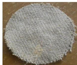
Fig.2: View of the Jute Geotextile Sheet
