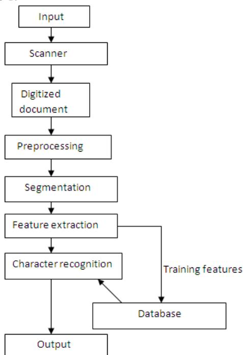
**Fig. 1** Block diagram of recognition system
