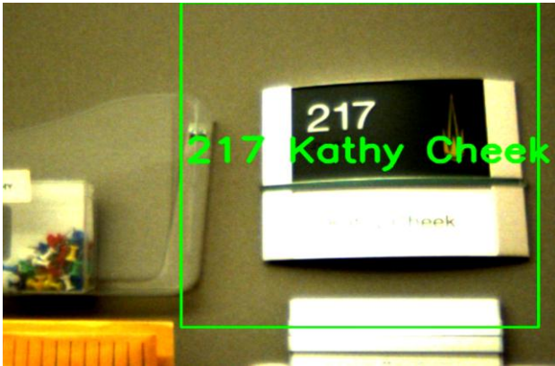
Fig 3: An example of an image used to generate a measurement of a door sign landmark. The text read by the OCR program is displayed.
