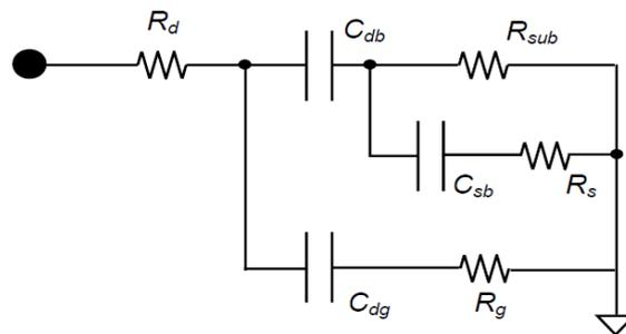
**Figure-2:** A compact RF model of gate-grounded MOSFETs.
