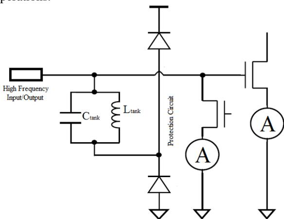
**Figure-7:**  $S_{21}$  ESD Isolation scheme with an LC-tank
