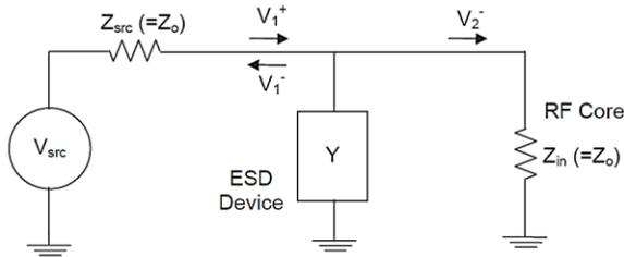
**Figure-3:** A two-port model of an HF Input/Output with an ESD protection device. (Y represents the ESD protection device)
