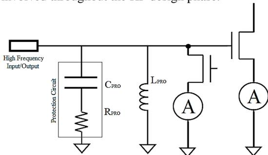
**Figure-6:** ESD cancellation scheme with an additional inductor
