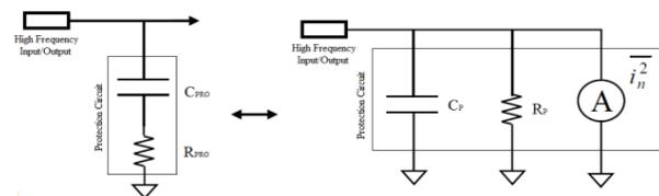
**Figure-1:** A simplified model of ESD protection circuit and its parallel configuration
