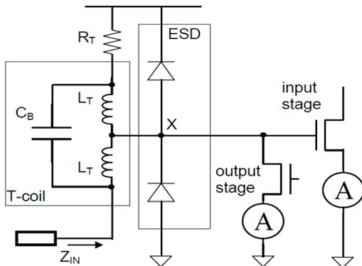
**Figure-9:** T-coil network for ESD protection
