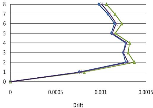
**Figure 8** Relative displacement profile of stories, a 8-storey structure, Northridge earthquake, damping ratio of 25%
