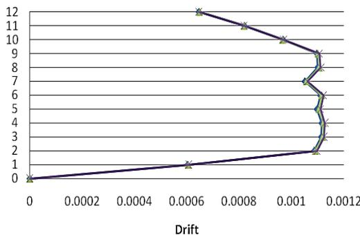
**Figure 9** Relative displacement profile of stories, a 12-storey structure, Northridge earthquake, damping ratio of 15%
