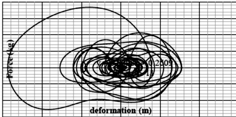
Figure 3 A sample of force-displacement curve of a viscous damper
