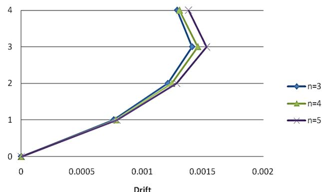
**Figure 5** Relative displacement profile of stories, a 4-storey structure, Northridge earthquake, damping ratio of 15%
