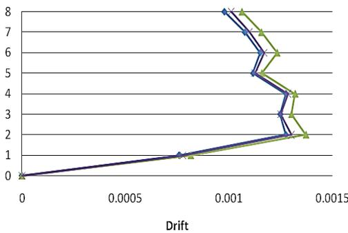
**Figure 7** Relative displacement profile of stories, a 8-storey structure, Northridge earthquake, damping ratio of 15%
