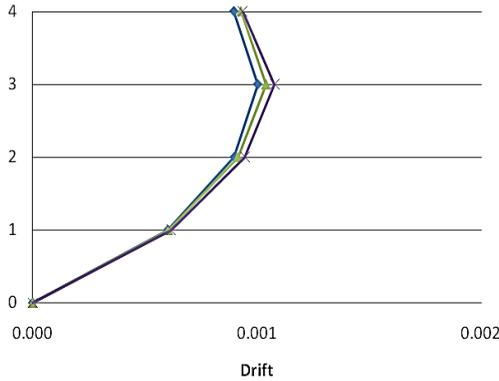
**Figure 6** Relative displacement profile of stories, a 4-storey structure, Northridge earthquake, damping ratio of 25%
