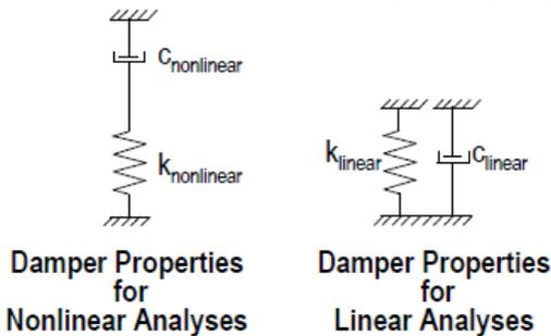
Figure 1 Damper element in SAP2000 software
