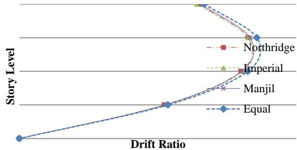
**Figure 11** Relative displacement profile of stories, a 4-storey building, Northridge earthquake, damping ratio of 15%
