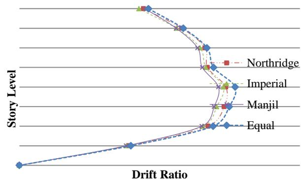
**Figure 12** Relative displacement profile of stories, an 8-storey building, Northridge earthquake, damping ratio of 15%
