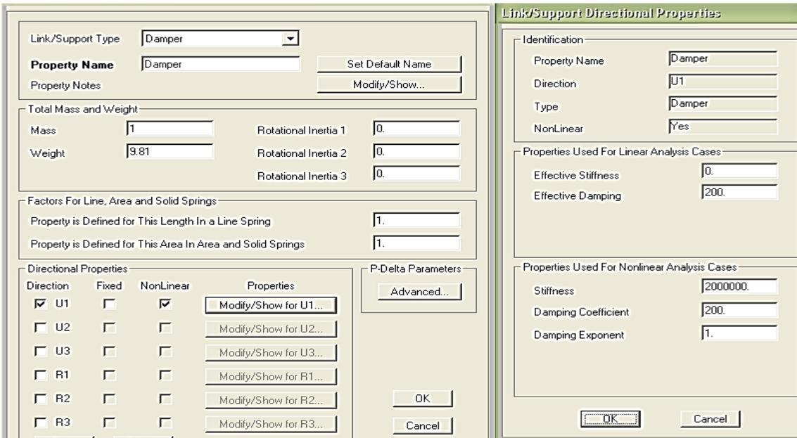
Figure 2 How damper element is modeled in SAP2000 software
