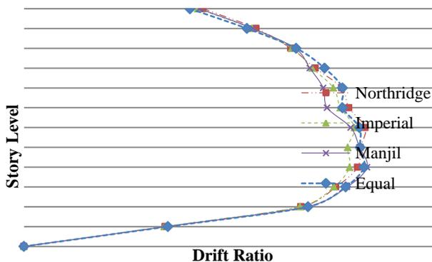
**Figure 13** Relative displacement profile of stories, a 12-storey building, Northridge earthquake, damping ratio of 15%
