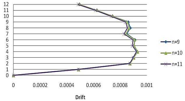
**Figure 10** Relative displacement profile of stories, a 12-storey structure, Northridge earthquake, damping ratio of 25%
