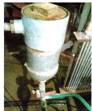
Figure 2.2: Air and water separator
