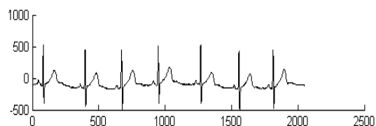
Fig. 5 Denoised ECG using hard filter with Visu rule
