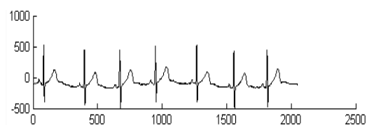
Fig. 6 Denoised ECG using soft filter with Visu rule
