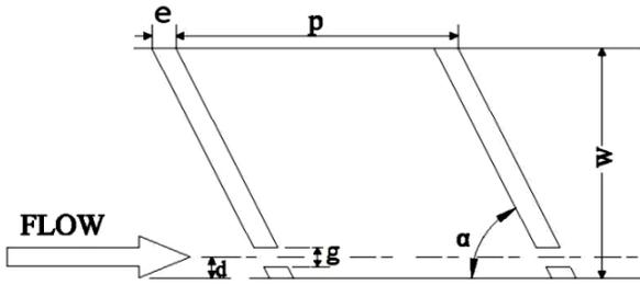
Figure 2: Schematic of roughness geometry of an inclined rib
