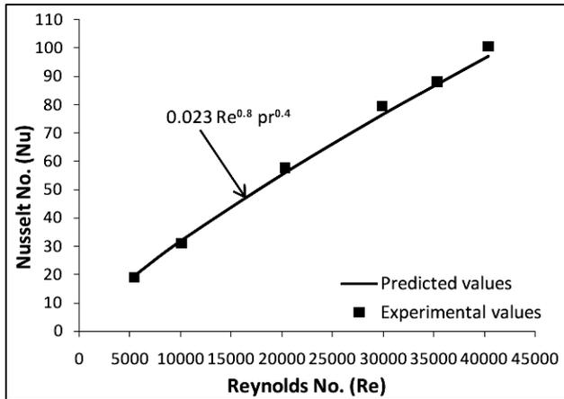
Figure 3: Comparison of experimental and predicted values of Nusselt number for smooth duct
