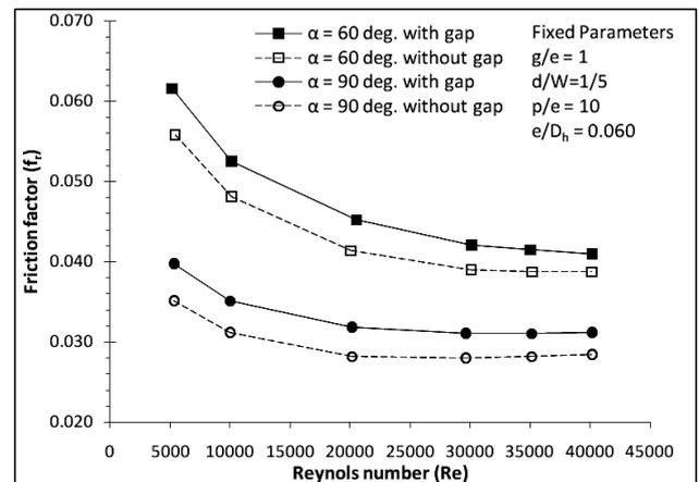
Figure 7: Variation of friction factor with Reynolds number for different cases
