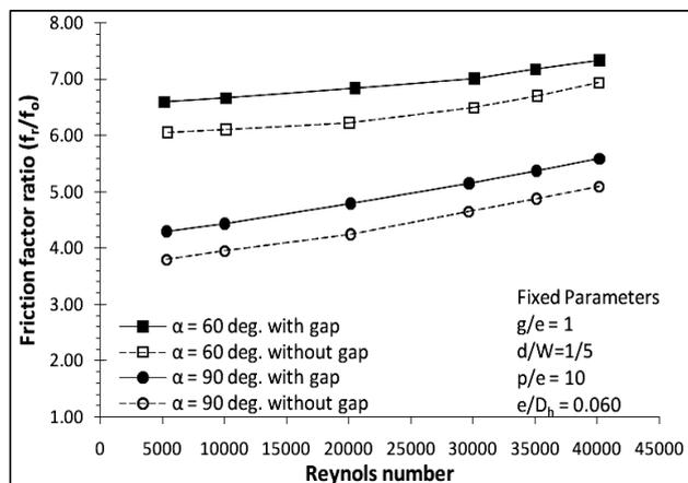
Figure 8: Variation of Friction factor ratio with Reynolds number for different cases
