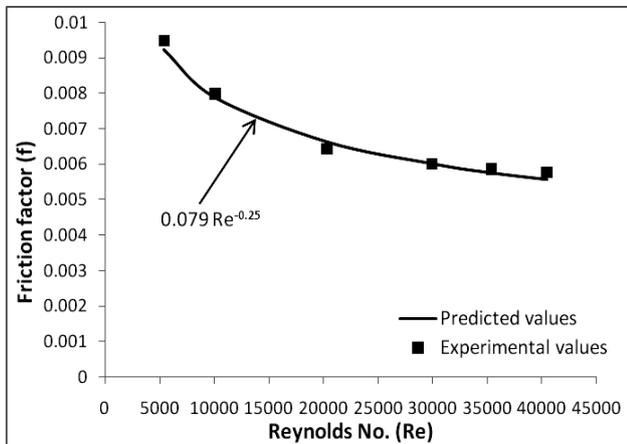
Figure 4: Comparison of experimental and predicted values of friction factor for smooth duct
