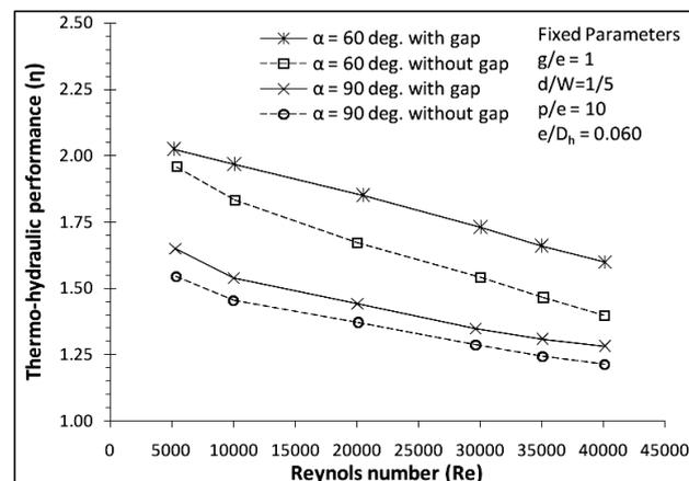
Figure 9: Variation of Thermo-hydraulic performance with Reynolds number for different cases
