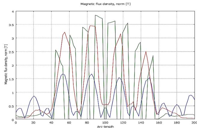
Fig. 5 Magnetic Flux Density for Primary, Secondary and Air-gap domain of Chamfered Model of LIM.
