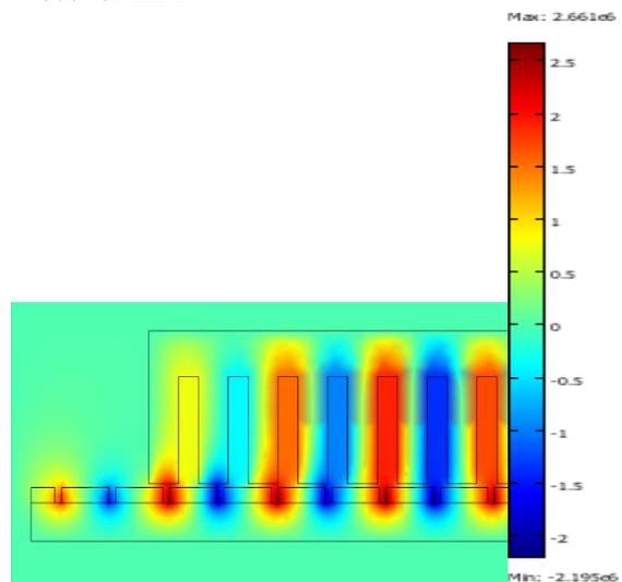
Fig. 8 Surface plot of Magnetic Potential of Simple Model of LIM
