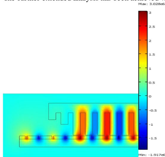
Fig. 7 Surface Plot of Magnetic Potential of Chamfered Model of LIM
