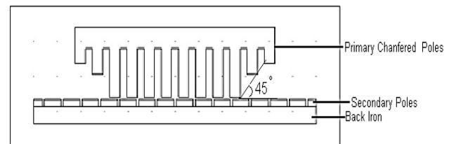
Fig. 2 Geometrical overview of Chamfered Model of LIM
