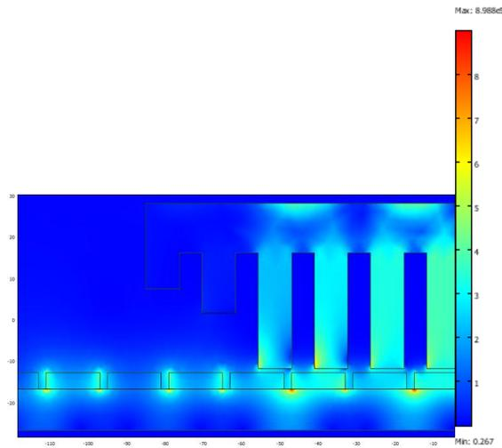
Fig. 3 Surface Plot of Magnetic Flux Density of Chamfered Model
