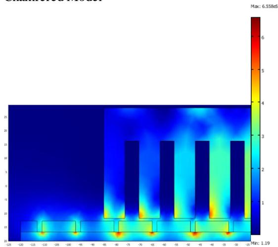
Fig. 4 Surface Plot of Magnetic Flux Density of Simple LIM
