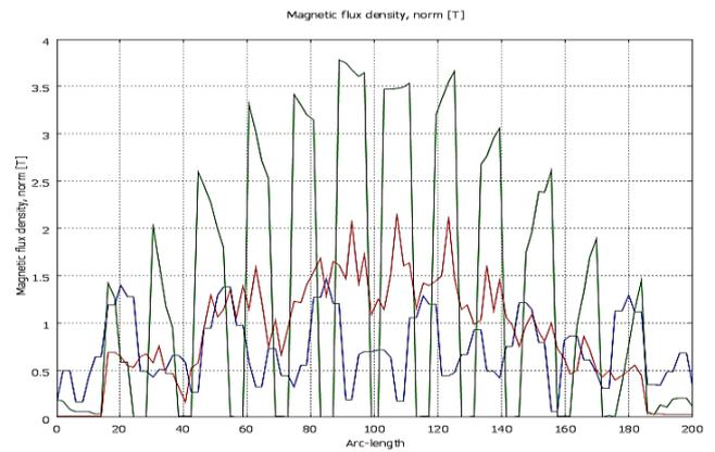
Fig. 6 Magnetic Flux Density for Primary, Secondary and Air-gap domain of Simple Model of LIM.
