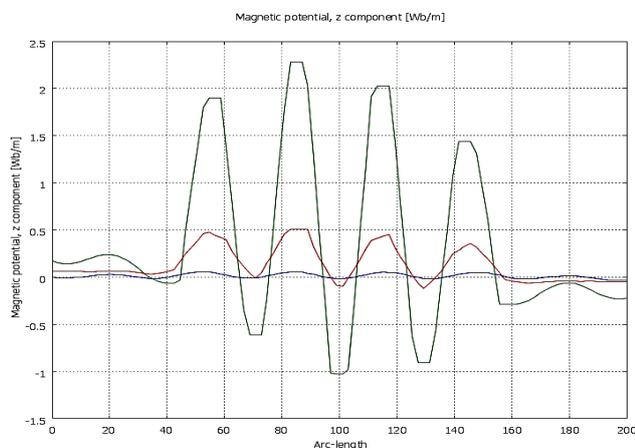
Fig. 9 Magnetic Potential graphs for Primary, Secondary and Air-gap domain of Chamfered Model of LIM.
