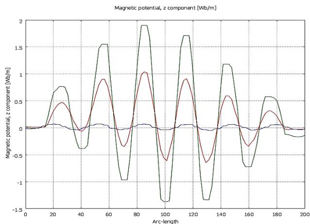
Fig. 10 Magnetic Potential graphs for Primary, Secondary and Air-gap domain of Simple Model of LIM.
