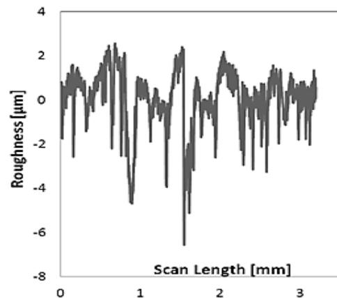
Figure 2 Roughness profile for the heating surface
