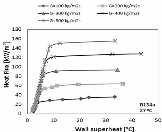
Figure 3 Boiling curve with 500 kg/m<sup>2</sup>s and at 27 and 32 °C saturation temperature
