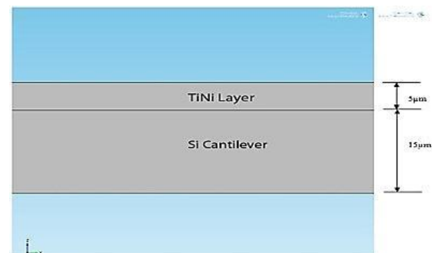
Figure 3.1: Shows the cross sectional view of the cantilever[4]
