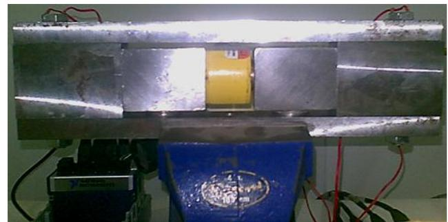
Fig 5. Experimental assembly subjected to shear load
