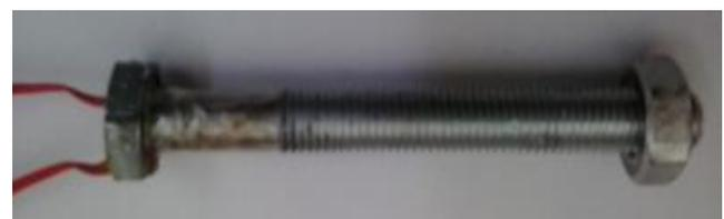
Fig 7. Bolt instrumented with two strain gauges
