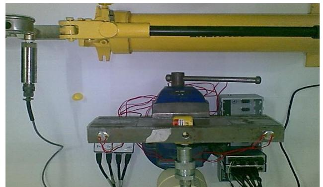
Fig 6. Manual hydraulic pump supplying the cylinder
