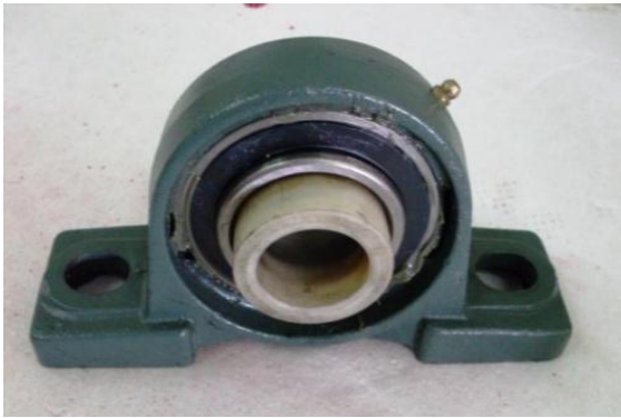
Fig 3. Nylon 6/6 Applied to Attenuate AE from the Rolling Element.
