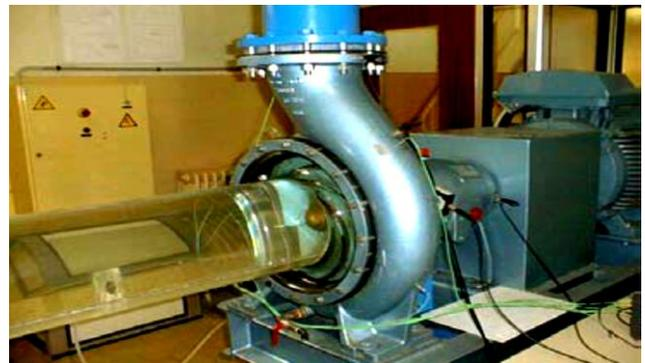
Figure 1: Experimental setup of the NS32 pump Asuaje (2005)
