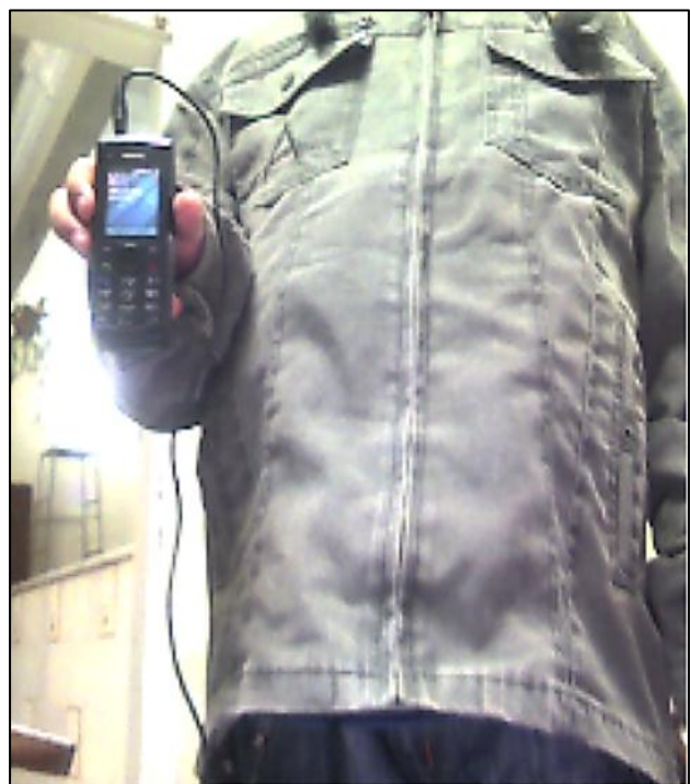
Figure 8 Mobile being charged by solar jacket
