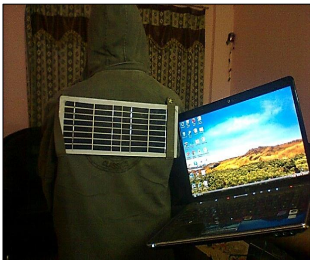
Figure 9 Laptop being charged by solar jacket
