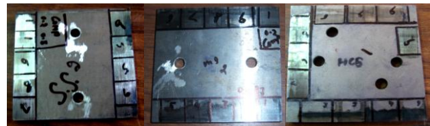
Fig.1 show presentation of machined work specimens: Stainless steel, Mild steel and High Chromium steel
