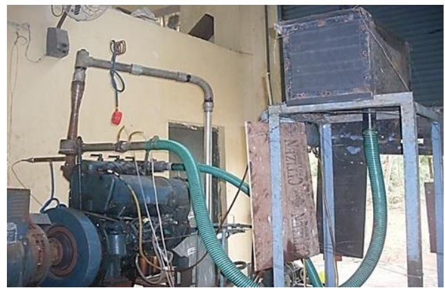
Fig 4.1 Experimental setup showing ejector connected to the diesel engine outlet
