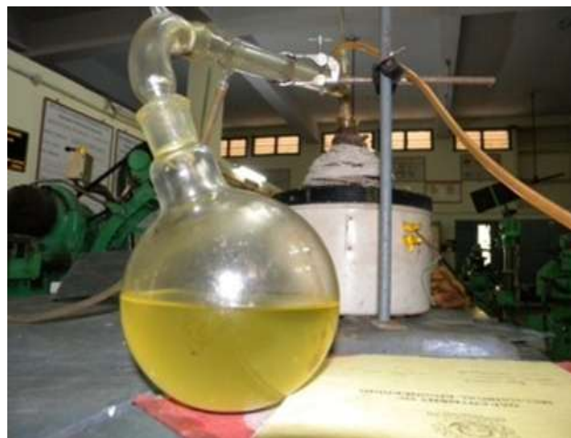
Fig.1 Experimental setup of fractional distillation to extract plastic petrol from liquid hydro carbons
