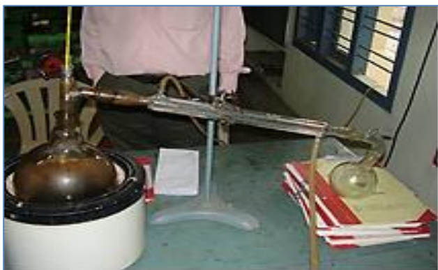
Fig.1 Experimental Setup of Fractional Distillation to Extract Plastic Diesel (PD) from Liquid Hydro Carbons Derived From Waste Plastic
