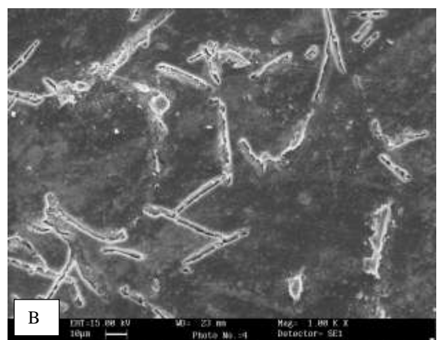
Fig.3a, b SEM micrographs of Al-6.23% Fe composite at different magnification
