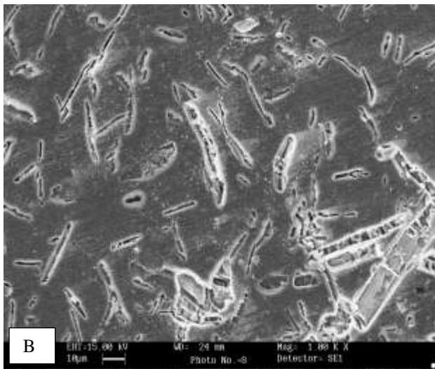
Fig.4a, b SEM micrographs of Al-11.2% Fe composite at different magnification
